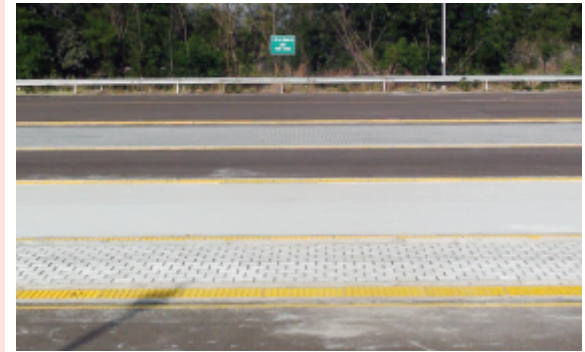
Cross Sectional View Showing Multi Friction Surfaces of ABS Test Track at NCAT, VRDE
