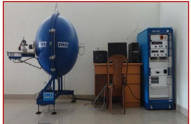
**c. Reflectance and Transmittance Measurement Equipment:** The system is designed for measurement of reflection and diffuse reflection at directional light incidences, for measurement of reflectance of mirrors, for measurement of transmittance and diffuse transmittance and diffuse transmittance at directed light transmittance.
