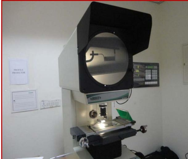
**d. Profile Projector:** The profile projector projects and magnified profile image of an area or feature of a work piece on to a screen, most commonly using diasopic illumination. Dimension can be measured directly on the screen or compared to a standard reference at the correct magnification.
