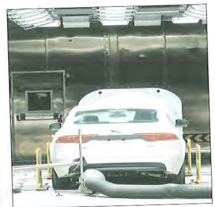
CLIMATIC VEHICLE TEST CELL AT ICAT
