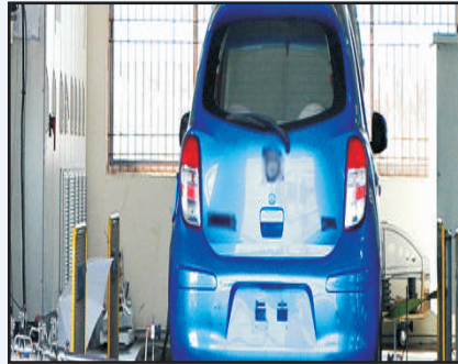
Mileage Accumulation Chassis Dynamometer (MACD) for 2, 3 & 4 Wheelers
